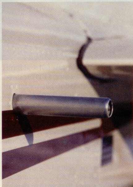
Serial number 5920, rolled out the door on January 5, 1948, and was the first of the 8 series equipped with the Silflex landing gear, also installed on Nievin's Luscombe (top). A handle installed on the empennage aids in parking the airplane (bottom).
