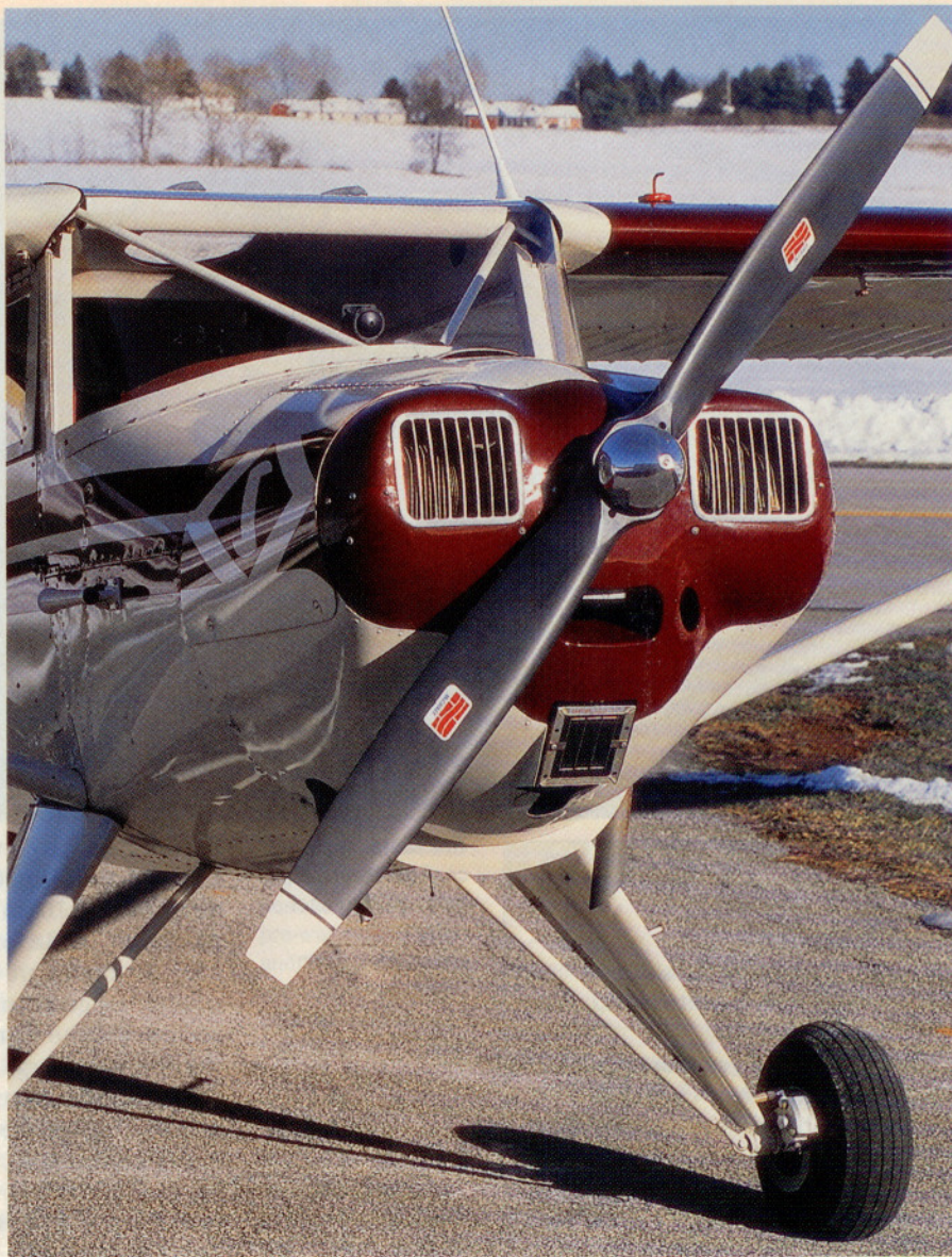
A venturi on the right side of the cowl (above) supplies vacuum pressure for the airplane's turn and bank gyro.
